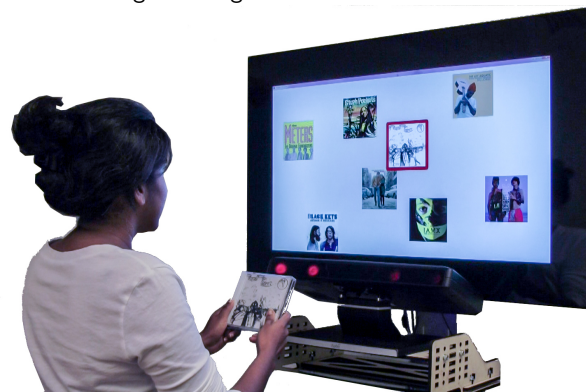
Figure 1: A user is interested in listening to a music album. She walks up to the in-store display, locates the album on the screen and follows its movement with her eyes. A sample of the music starts to play automatically.
