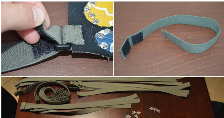
Fig. 2 This is a composite image of the modular strapping. The above images show how straps are attached to the RPWTB (top left), general strap design (top right), and the range of lengths provided (bottom)
