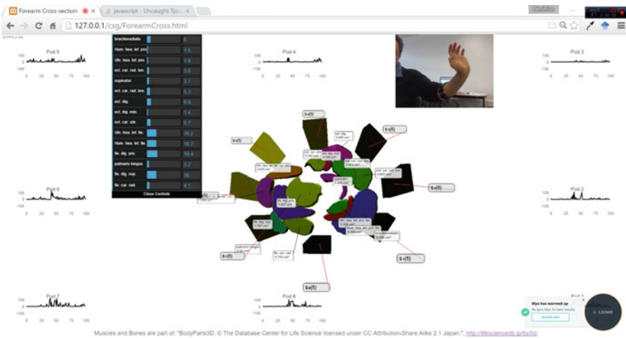
Fig. 10 A screenshot of the visualization software by Ververidis et al. (2016). In the middle of the screen, eight Myo electrodes are presented together with the relevant arm muscles (cross-sectional volume). (Created with permission from Dimitrios Ververidis n.d.)
