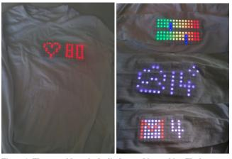
Figure 1. The wearable on-body display used in a t-shirt. The heart rate visualized on the chest (left) and a progress bar, weather information, and e-mail notification on the forearm (right).
