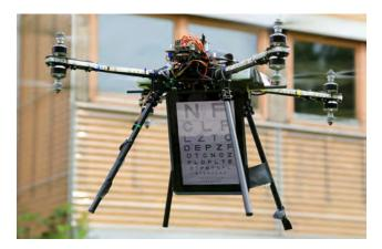
Figure 4: Midair display prototype with Snellen chart.
