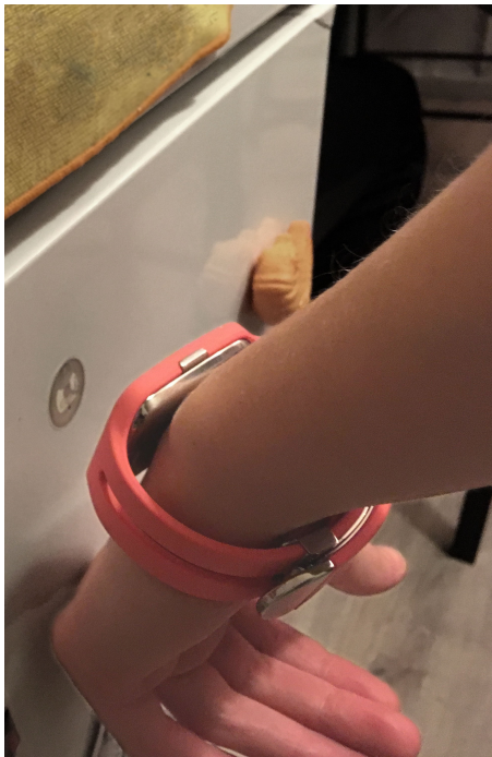
Figure 1: Logging Process: Participant accessing the fridge and logging the interaction by reading the respective NFC tag using the smartwatch.
