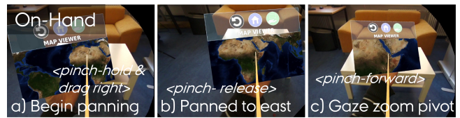
Figure 11: The Map Viewer has continuous pan & zoom, via a pinch-dragging into the gaze-based zooming pivot.
