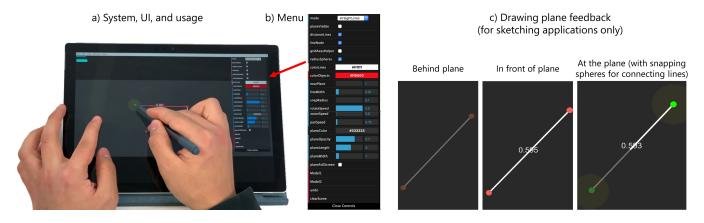
Figure 5: Our application prototype explores two-handed pen and touch tools (a). The menu allows to customise the GUI and select particular tools (b). Sketching happens on a transparent drawing plane in front of the screen-space, which is indicated through brightness feedback (c).
