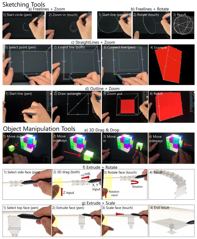
Figure 6: Techniques implemented in our application, empowering the user in the manipulation of 3D content. The top half presents applications for sketching (a-d), and the bottom half for 3D object transformations (e-g).
