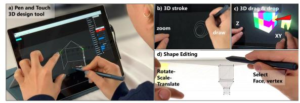
Figure 1: *Bi-3D* is an interaction concept to create and manipulate 3D objects and sketches. E.g., to edit shape points (a), draw a 3D stroke (b), 3D drag & drop an object (c), or scale shape (d) – enabled by a dynamic coupling of pen and touch in both hands.
