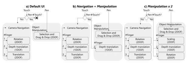
Figure 3: High-level input state models. (a) A simplified model of a typical 3D UI with separable pen and touch, and two new models where touch input enhances the pen's manipulation with (b) and without (c) parallel navigation operations.
