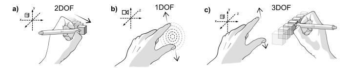
Figure 2: The Bi-3D concept exploits bi-manual gestures for extension to 3D object interaction. For example, individually, a system can support a 2D drag & drop via pen (a) and a 1D pinch-to-zoom gesture to change camera depth (b). In combination, they offer possibilities to extend to 3DOF operations, useful for 3D transformations such as 3D drag & drop (c).
