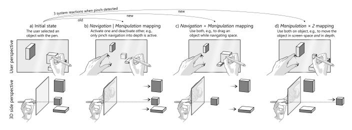
Figure 4: Navigation/Manipulation Mappings: The user begins with selecting a target (a). If the user engages a pinch gesture, typically only one mode is active (b). We propose two new mappings: users can drag an object via pen while navigating in 3D, which represents an intuitive extension from 2D to 3D (c); and users apply both pen and touch commands to one object for more expressive input (d).
