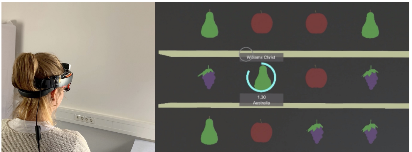
Fig. 9. Shopping: gaze, particularly dwell-time, plays two crucial roles: it can modulate the amount of augmented information displayed in response to users' attention (e.g., show the item cost); and allow users to interact with the item being gazed at (e.g., to "add to cart").
