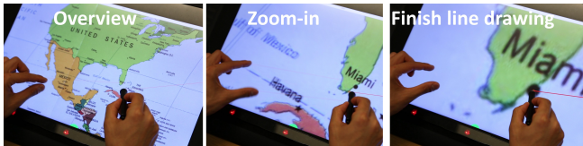
Figure 3: Pen-touch: While users are drawing a line, users can zoom into the pen’s position and then precisely finish the line drawing.
