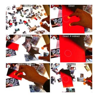
Figure 11: Locally zoom directly, globally zoom indirectly: users can globally zoom the canvas with indirect touch (a-b), locally zoom objects with direct touch (c-d), and immediately return to global zooming (e-f).
