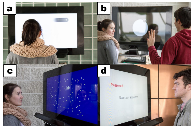
Figure 1: Pursuit calibration is based on moving targets (a), tolerates interruptions (b), can blend with application tasks (c) and calibrate users even when they are not aware (d).
