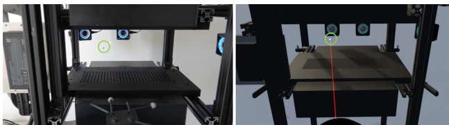
Figure 11: In the LeviShooter game, the player aims at the levitating particle (marked with a green circle), using a lasergun. The goal is to successfully hit the particle, as often as possible, while with every hit, the particle velocity increases.
