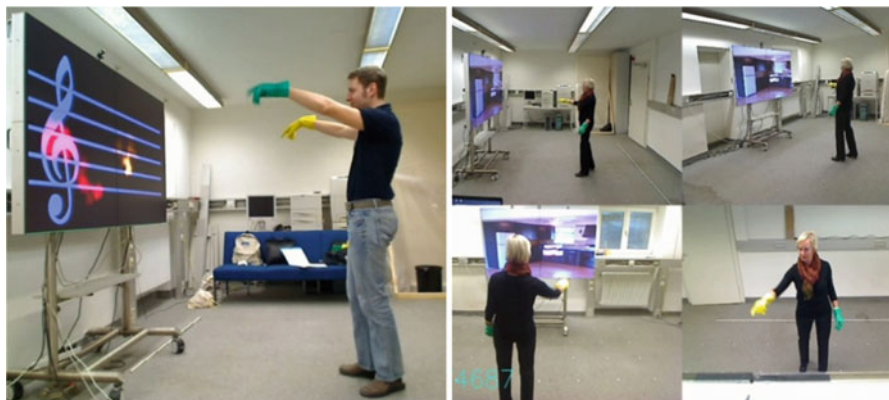
Fig. 16.7 Recordings of the user study on our interactive musical advertisement. In the left image the user controls a red particle visualization with one hand, and a yellow particle visualization with the other hand. The left hand is used to control the rate of played notes, and the right hand controls the pitch. In the right image a test run with one-hand control is seen
