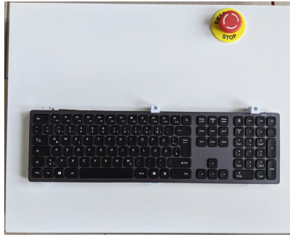
(b) Top view of our finished prototype. The keyboard is fixed with 3D-printed clamps and an emergency button is placed in the right corner.
