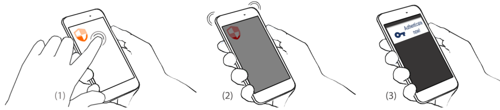
Figure 1: We propose to use indicators to communicate both the current device confidence level ( DCL ) and the need for re-authentication for continuous implicit authentication systems on mobile devices: (1) a long term indicator illustrates the current DCL and its development over time via a task bar icon, and (2) a short term indicator announces an upcoming re-authentication via darkening the screen. Our system also allows for (3) voluntary re-authentication to avoid system-side locking of the device.
