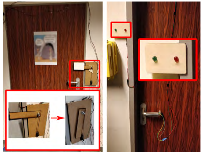
Figure 4. Left: The back view of the door. The mechanical door lock was controlled over a wireless network. Right: The front view of the door. Additional feedback regarding the success of an authentication attempt was provided by coloured lights at the front side. The green LED on the left indicates success, the red LED on the right failure.
