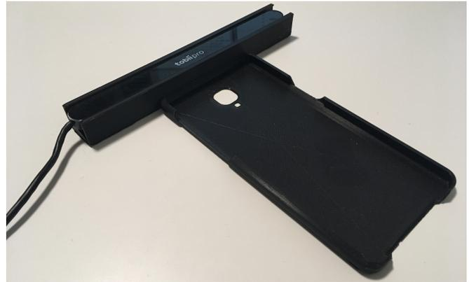
Figure 2: The 3D-printed phone case with the attached Tobii Pro Nano eye-tracker.
