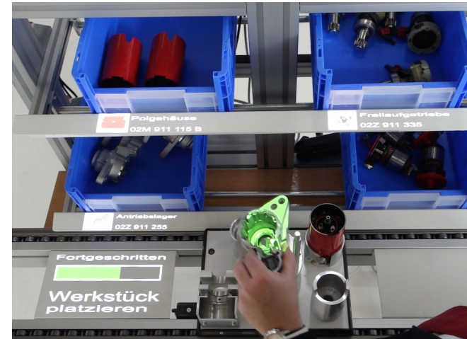
Figure 1: Assembly of an engine starter using in-situ projections. Assembly instructions are displayed into the field of view of the worker. Image source: [8].
