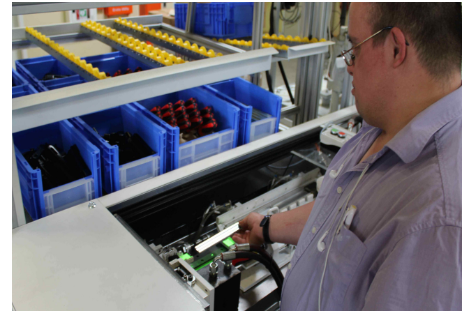
Figure 3: Worker assembling a clamp in a sheltered work organization using in-situ projection assistance. Continuous in-situ assembly instructions were perceived as helpful.
