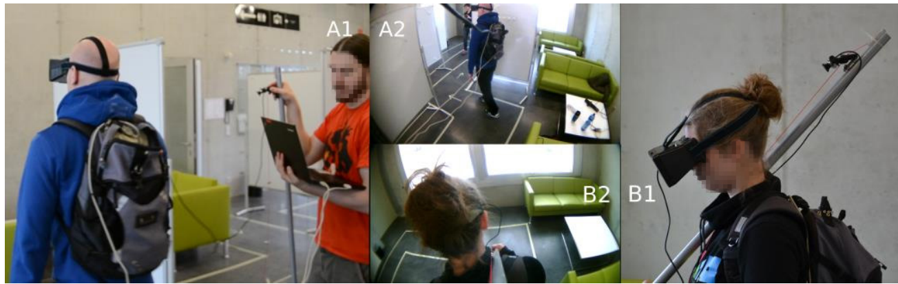
Figure 1. The WOz approach (A1) allows the participant to see their full body (A2). The stick approach (B1) enables a better control of view (B2).
