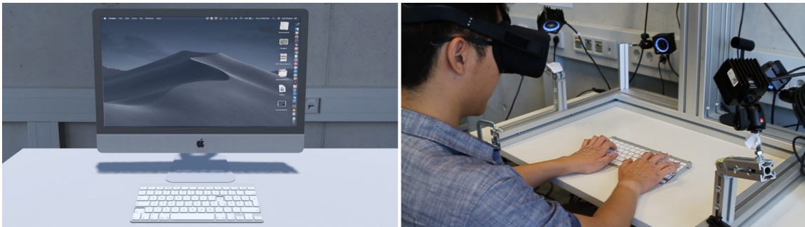
Fig. 1. Left: A virtual office workspace resembling the physical exemplar (built with Unity 3D Engine). Right: Stationary apparatus comprising a workstation, VR headset, and accurate optical tracking system to enable text input in virtual reality.
