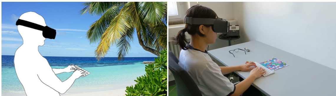
Fig. 2. Left: Inspiring virtual office that is designed according to the employees’ needs. Right: lightweight, mobile setup comprising a smartphone, VR viewer, and physical keyboard to enable text input in virtual reality.
