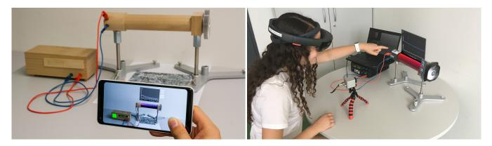
Figure 1: A person uses our prototype to understand thermal flux in a physics lab experiment. Users can either use a smartphone (left) or HMD (right) to extend their sight by thermal vision. Virtual elements are an extension for non-functional setups to simulate a real experiment.
