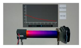
Figure 2: False-color representation of the metallic rod showing the thermal flux. Temperature changes can be observed in real-time using a smartphone or HMD.
