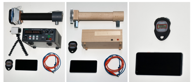
Figure 3: Entities for experimental assembly for all three conditions. (Left) real : Power supply, metal probe, thermal camera, wires, smartphone and stopwatch. (Center) replica : wooden power supply replica, wooden probe replica, wires, smartphone and stopwatch. (Right) virtual : smartphone and stopwatch.
