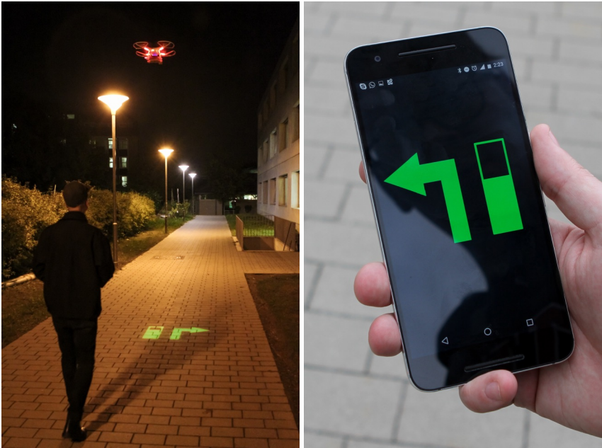
Figure 4.2: We conducted a user study comparing (left) projected in-situ navigation instructions to (right) traditional navigation instructions presented on a smartphone.
