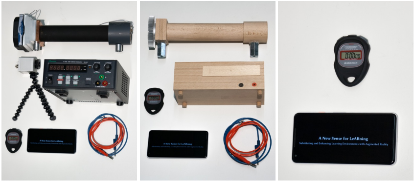
Figure 5.3: Entities for experimental assembly for all three versions. left) real : Power supply, metal probe, thermal camera, wires, smartphone and stopwatch. center) replica : wooden power supply replica, wooden probe replica, wires, smartphone and stopwatch. right) virtual : smartphone and stopwatch.
