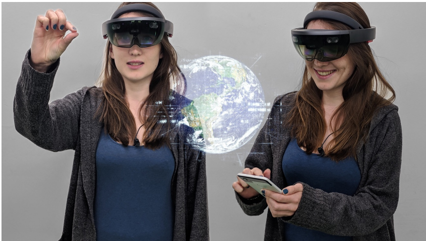
Figure 8.1: We conducted a user study comparing traditional mid-air hand gestures (left) to hybrid interaction with a smartphone (right) as in and output controller in Augmented Reality environments.
