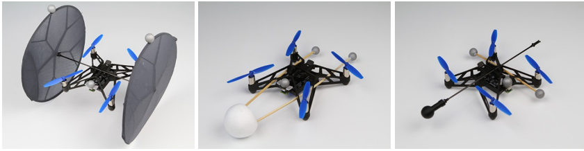
Figure 7.2: Quadcopter prototypes to deliver different types of feedback. (left) passive feedback, (center) active feedback, (right) haptic proxy feedback.
