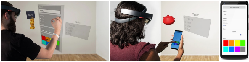
Figure 8.6: The conditions of the second experiment. Participants are either controlling the GUI via mid-air gestures (left), touch gestures on the smartphone or the GUI is displayed on the smartphone itself (center/right) while the task and elements are displayed in AR.
