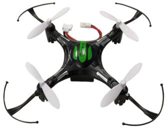
Figure 2: Quadcopter used as levitating tangible device.
