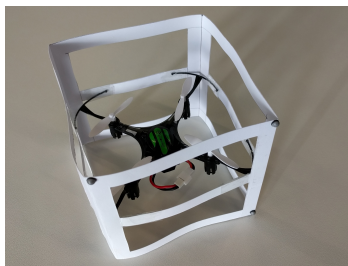
Figure 3: Quadcopter equipped with a cage to enhance tangible interaction.
