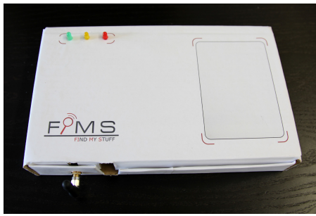
Figure 6: StarterKit with LEDs for visual feedback.
