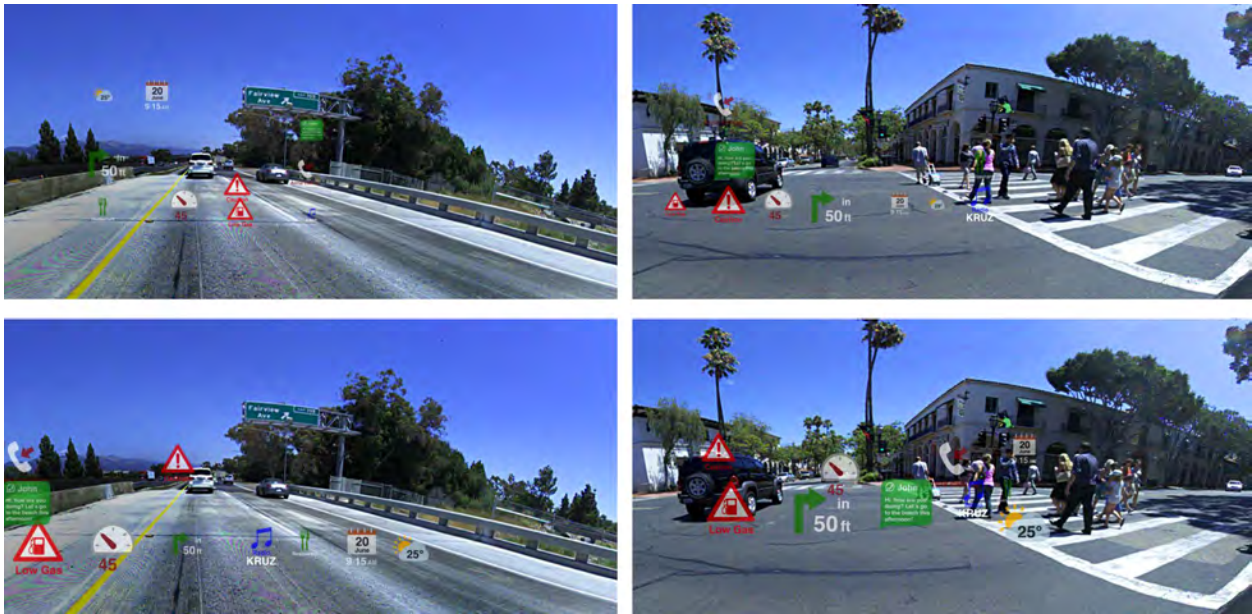
Figure 7. Examples of personalized layouts. The background shows the driving scene in which the final layout was created. Based on the AOIs (defined in figure 2), we would not recommend to use these layouts on the road.
