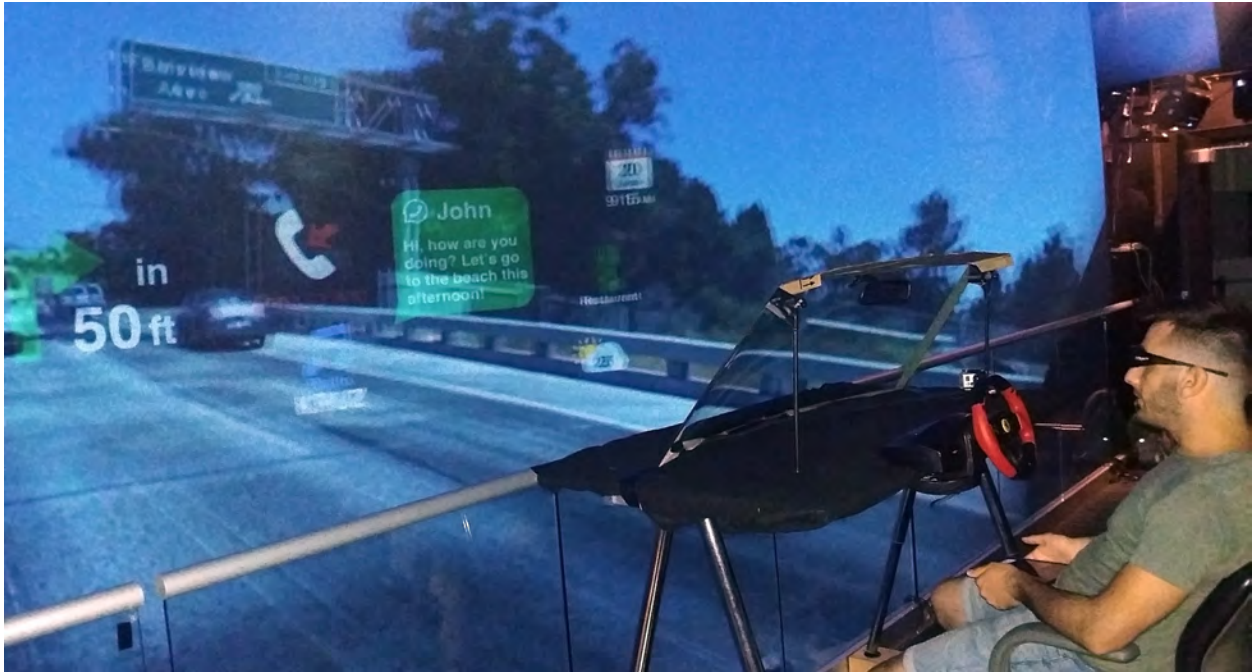
Figure 5. A participant creating his personal layout. The participant placed items within areas relevant for safe driving. Thus, we do not consider this layout safe.
