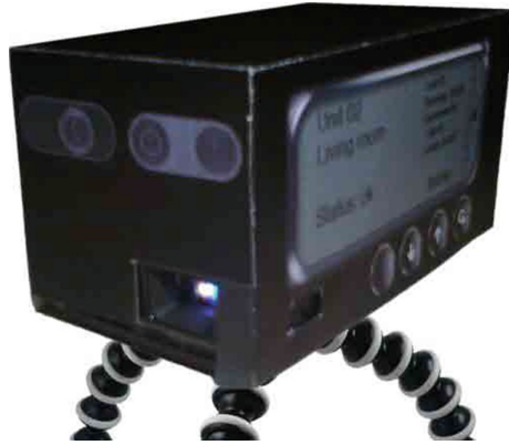
Fig. 2. Mock-up consisting of a projector inside a cardboard box mounted on a flexible camera stand
