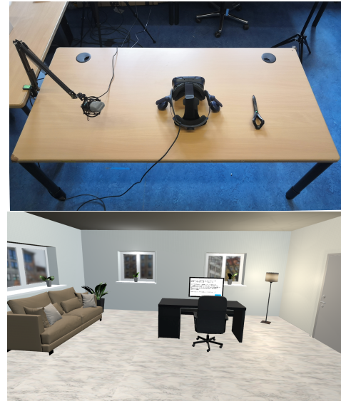
Figure 2: Real-world and virtual study environments. Top: Lab study set-up. Participants sat at a table that was exactly matched with the table in the virtual environment. A microphone was attached to the table, that was used to trigger avatar animations when certain keywords were detected. Bottom: The virtual environment. Participants sat on the chair, facing the computer screen.
