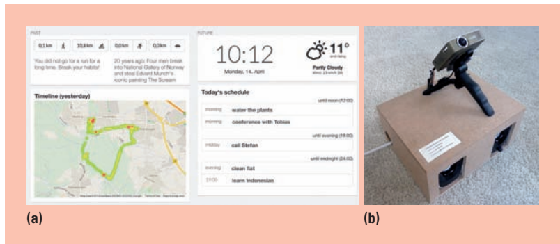
Figure 2. Memory display prototype. (a) The system dashboard shows a summary of movement data from the past, fitness goals, current weather information, and the day's schedule. (b) The physical prototype is a bedside device.
