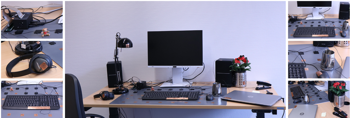
Figure 1: Act2Auth embeds authentication in the way in which users interact at a desk setup. Users of Act2Auth can authenticate by touching objects or the desk itself in a secret order similar to a password. To evaluate our concept, we built a prototype that applies capacitive sensing to daily life objects and conducted an exploratory user study ( N = 8 ).
