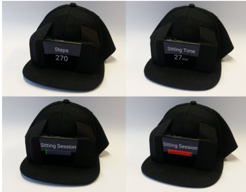
Figure 2: Hat Tracker Prototype, showing the 3 different display modes supported – step count (top left), total sitting time (top right), sitting time bar chart (bottom). The display mode was selected at random every minute.
