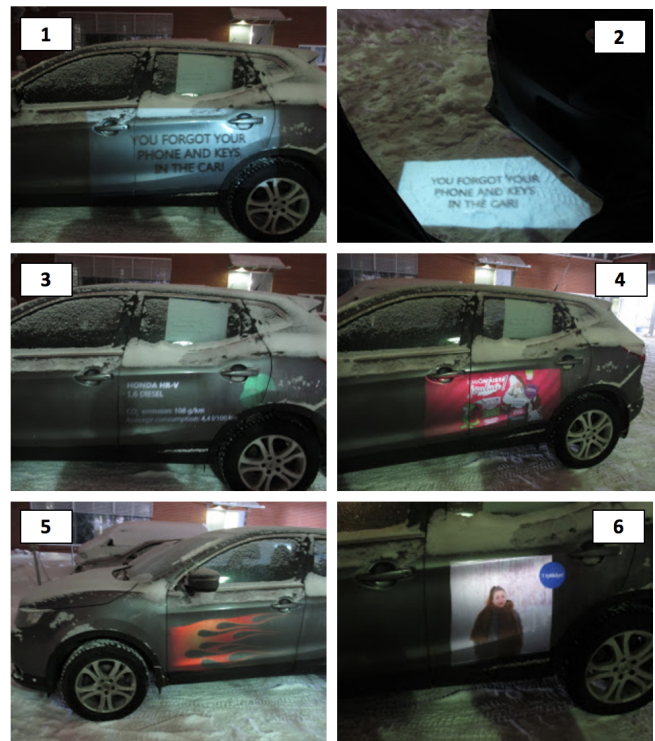
Figure 4. Car external surface display concepts. 1&2) Warning driver of forgotten keys. 3) Real-time environmental information. 4) Dynamic advert (e.g. dependent on parking location). 5) Changeable aesthetic surface patterning. 6) Driver's social media post displayed on car surface.
