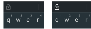
Figure 4. The private mode button, added to the left of the word suggestion bar. The symbol shows whether it is inactive ( left ) or activated ( right ). No data is collected in private mode. We chose a symbol instead of text to save space on the keyboard. To ensure that functionality and meaning was clear to all participants, we explained the button and private mode in the initial study meeting.
