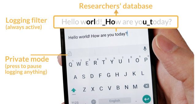
Figure 1. Our ResearchIME keyboard app for free text typing studies in the wild, based on Android's open source keyboard. Logged events are sent to the researchers' server. However, data is filtered on the device to avoid logging readable text. The figure shows a random n -gram filter; non-redacted data is highlighted. In addition to the filter, a private mode button allows users to pause logging entirely.
