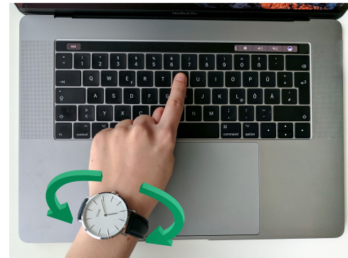
Figure 1. We propose to extend keyboard shortcuts with arm and wrist rotations gestures, performed while pressing down a key. The figure shows left/right wrist rolls. The user’s rotation angles can be used, for example, for continuous control, such as changing the volume.
