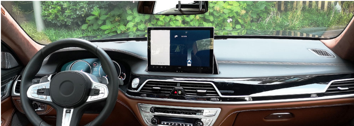
Fig. 3. Prototype mounted in front of the CID. The system detects emotional states using a camera in the bottom frame of the device.
