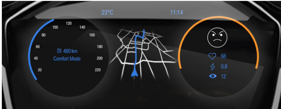
Fig. 1. Our prototype of an affective interface showed driver state data in the instrument cluster. Focus group participants (US and Germany) expressed general curiosity and potential for improving driver safety, but also concerns regarding paternalism.
