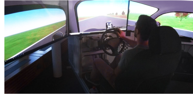
Figure 2: User study setup: participants experienced a driving simulation while they interacted with the face recognition system. A smartphone positioned on top of the steering wheel showed the music player and direct feedback.
