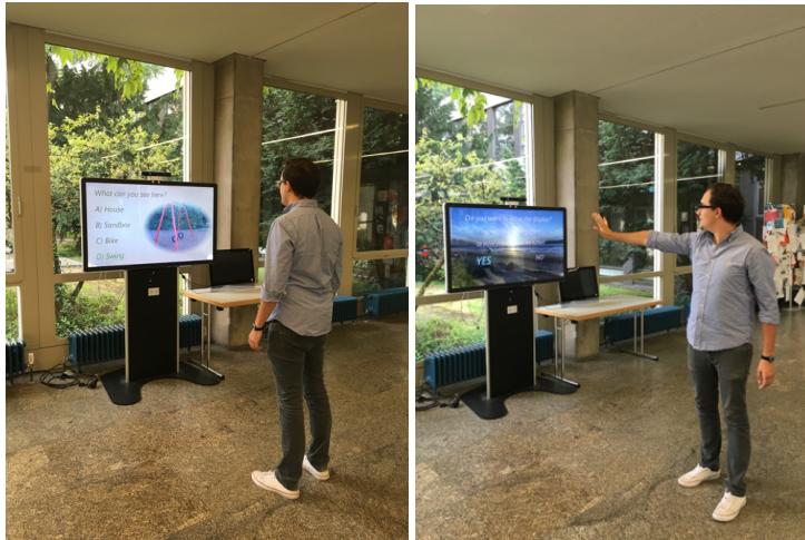
Fig. 3. To prove the concept we deployed the display in a University setting. The display shows a quiz (left). As the system thinks the user is about to leave, users are shown a prompt (right), asking them to confirm whether they are indeed about to leave or not. Users can provide feedback by hovering with their hand over yes/no buttons.
