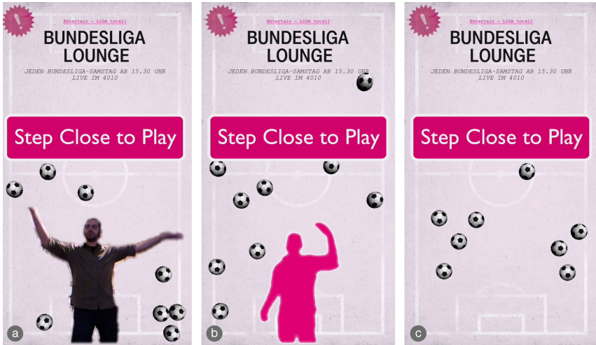
Figure 8.5: User Representations: Mirror (a), Silhouette (b), and No-Representation (c). All three representations were tested in an ‘attract loop with call-to-action’ as well as in an ‘inadvertent interaction’ version. In this figure, the corresponding attract loops (a video of somebody stepping close to the display and starting to interact) are shown. In the inadvertent interaction condition, the person in front of the display is shown in the same representation, just without the call-to-action (‘Step Close to Play’).
