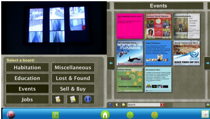
Figure 9.4: Digifieds Display Client: The display client shows an overview of the different views on the left, the active view, containing the actual digifieds, is located on the right.
