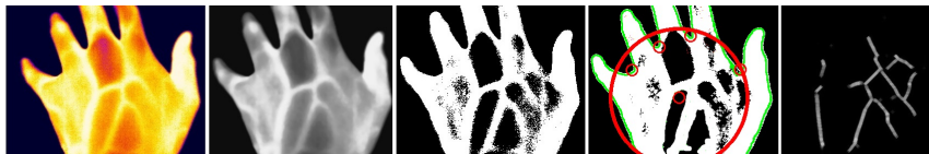
Figure 4.17: Veins extraction algorithm.
