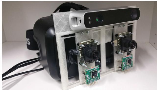
**Figure 1:** Proof of Concept prototype consisting of Head Mounted Display with augmented RGB, Depth and Thermal Cameras.
