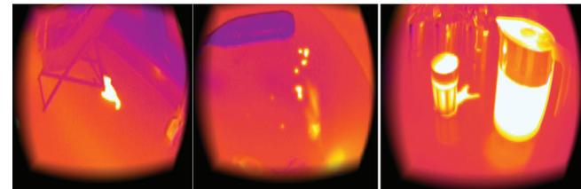
**Figure 4:** Sample Images from thermal camera showing hidden cat-shaped bottle, leakage of water bottle and level of water inside a kettle.
