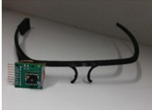
**Figure 3:** Miniature FLIR lepton thermal camera attached to a 3D printed glass, envisioning the potential form factor.
