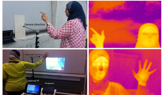
Figure 1. (top) the outdoor setup with the thermal view of tile as the reflective surface (bottom) the indoor setup with the thermal view of glass as the reflective surface.
