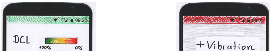
(c) Color-changing status bar with a color range based on a traffic lights approach. The color depends on the current DCL. When a reauthentication is necessary, the screen starts to dim-out gradually and the phone vibrates.
