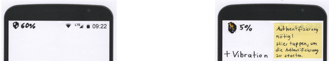
(a) Symbol and device confidence level (DCL) in the status bar. When a reauthentication is necessary, the symbol changes and a notification with vibration appears.
