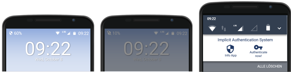
(a) Long Term: Symbol and percentage of DCL in the status bar. (b) Short Term: Dimmed screen with optional vibration. (c) Notification: Can be used for voluntary reauthentication.
