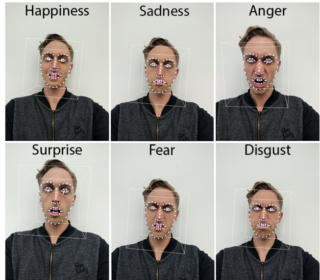
Figure 3: Six basic emotions defined by Ekman et al. [11, 16]. A modified version of OpenFace [3] uses the front camera to detect landmarks on faces as indicator for emotions.
