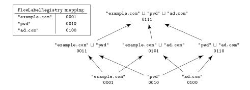
Fig. 1. The FlowLabelRegistry mapping three JavaScript strings used as security principals to unique bit positions. These principals form a lattice of security labels, represented as bit vectors.
