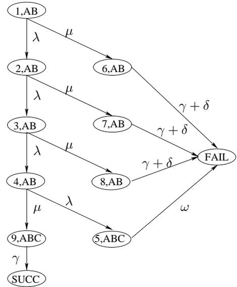
Fig. 5. Product automaton  $\mathcal{M}^\times = \mathcal{M} \times A_\pi$  for checking validity of  $\Phi_3$
