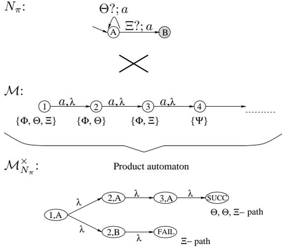
Fig. 6. Incorrect product automaton for  $\varphi_{im}$
