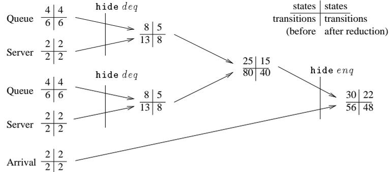
Fig. 3. Compositional reduction of the example queueing system
