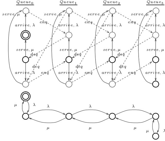
**Fig. 2.** Top: The LTS for the example queueing system. Bottom: The corresponding CTMC
