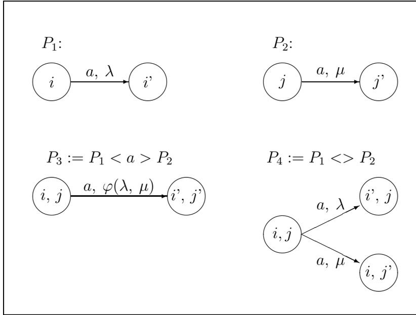
Figure 6: Composition of processes, synchronisation and interleaving
