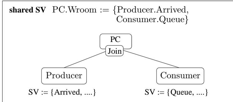
Figure 3: Hierarchic composition of the PC submodels via *Join*
