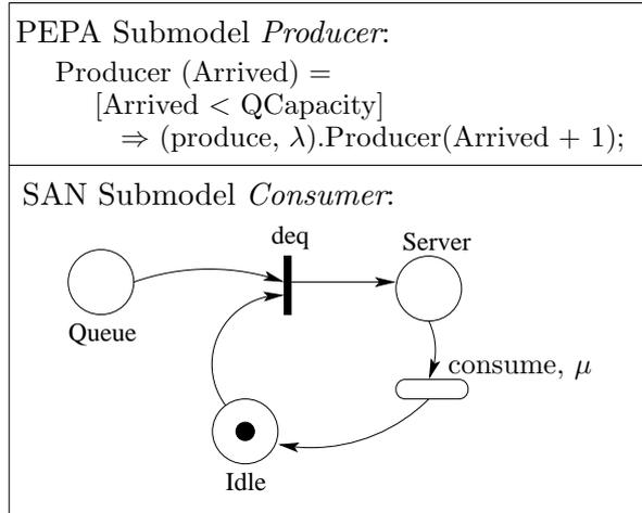
Figure 2: PC system consisting of a PEPA and a SAN submodel
