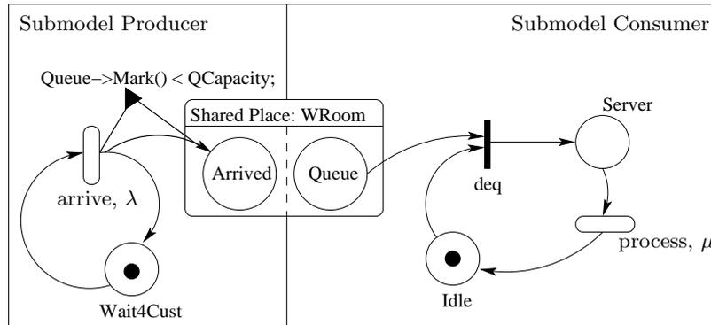
Figure 7: PC system modelled by two SAN submodels
