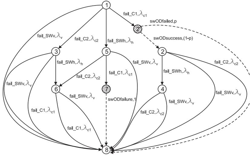
Figure 3: State space of the small reliable system (using Kececioglu's general switch model)
